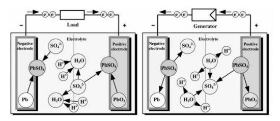
Gambar 2. 12 Charging dan Discharging Lead-Acid Battery (Quaschning, 2016)
