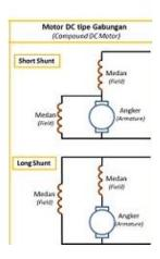
Gambar 2. 4 Rangkaian Motor DC Compound
