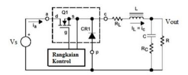
Gambar 2. 21 Rangkaian DC Chopper Step-Down
