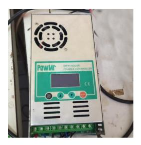
Gambar 2. 19 MPPT (Maximum Power Tracking)
