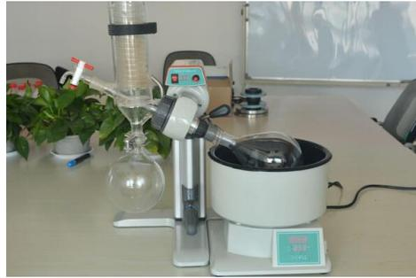
**Gambar 2.2** *Rotary evaporator*
