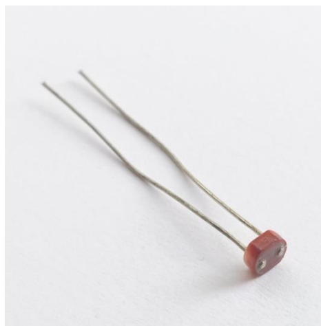
Gambar 2.2 Sensor LDR ( Light Dependent Resistor )
