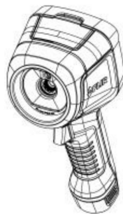
Gambar 3. 4. Mechanical drawings pemindai termal FLIR-E40
