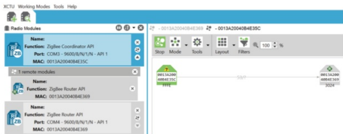
Fig. 8. Configuration of XCTU to determine the status of the remote module and local module.
