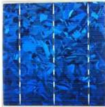
Gambar 2.7 Panel Surya *Poly-crystalline*
