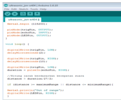
Figure 11. The syntax of communication program between sensor and Arduino-Uno.
