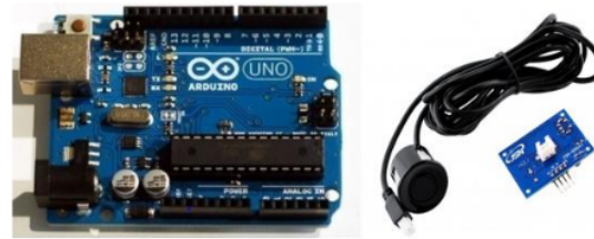
Figure 1. Arduino-Uno circuit board and JSN-SR04T sensor [6].
