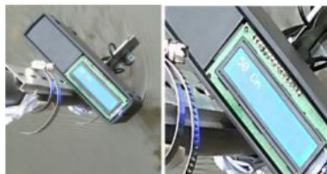
Figure 14. Water level testing at 50cm.
