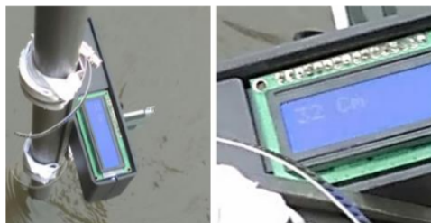
Figure 13. Water level testing at 32cm.
