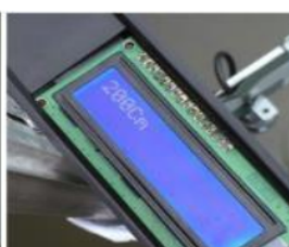
Figure 18. Water level testing at 200 cm.
