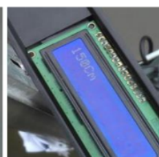
Figure 17. Water level testing at 150 cm.
