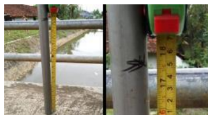
Figure 19. Validation of measurement result by measuring pole.
