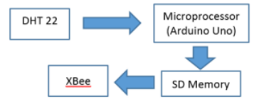
Fig. 3. Schematic batch process on the sensor node.
