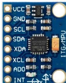
**Gambar 2.9** Sensor MPU-6050
