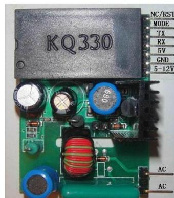
Gambar 2.7 Modul *Power Line Carrier* (PLC) KQ330
