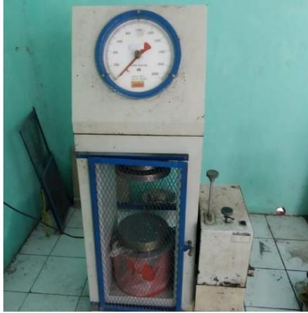
**Gambar 3. 13** *Compression Testing Machine (CTM)*
