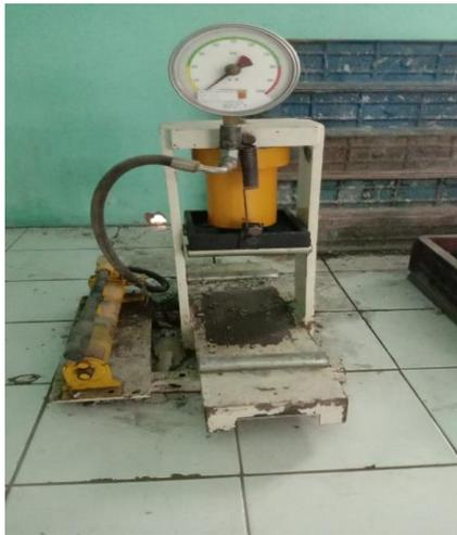
**Gambar 3.18 Hidraulik Jack**
