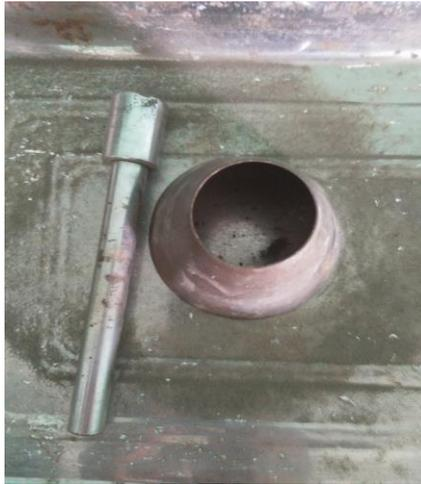
**Gambar 3.10** *Sand Conical Mould*
