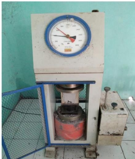
**Gambar 3.7** *Compression Testing Machine*
