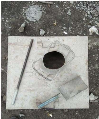
**Gambar 3.3** *Slump Test*
