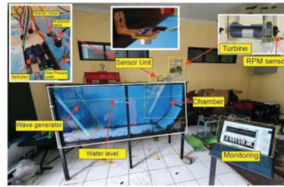
Fig. 4. Prototype OWC test rig in laboratory-scale
