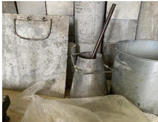
**Gambar 3.10** *Kerucut Abrams*
