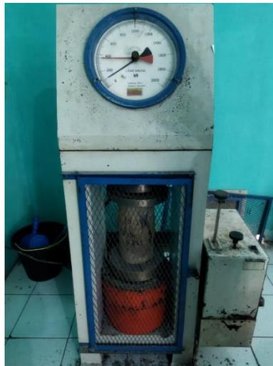
Gambar 3.14 *Compression Test Machine*
