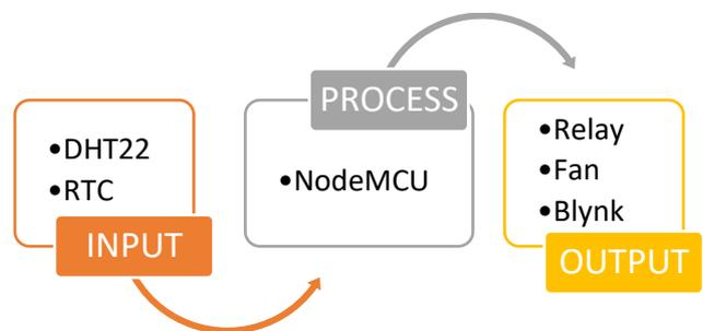
Fig. 2 Block Prototype Diagram
