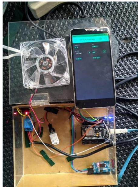
Fig. 10 The temperature is below 30°, and the fan does not turn on.
