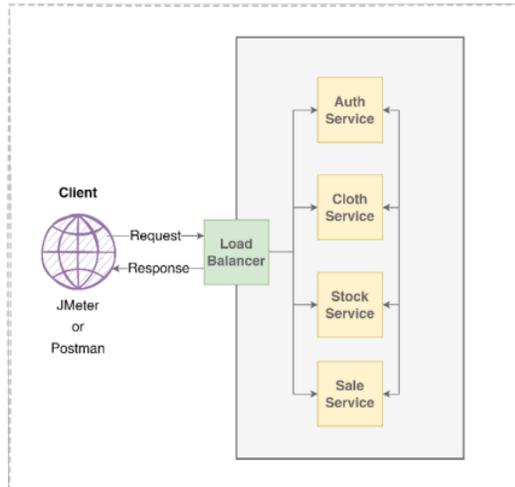
Fig. 3. API-Driven Architecture Communication Process in Microservice
