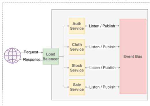
Fig. 1. Event-Driven Architecture Communication Process in Microservice
