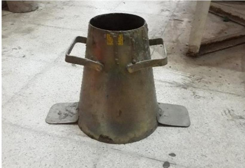
Gambar 3. 14 Kerucut Abrams
